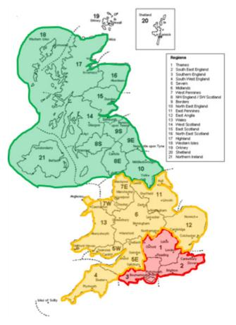
Figure #1-1: Risk zoning from geographical location, based on average external temperature and average solar radiation between May and September (data and zones from SAP 2012 version 9.92, October 2013; These are unchanged in draft SAP 10, 2018).
