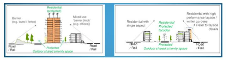
Figure #3-3: Examples of site layout mitigation measures.
