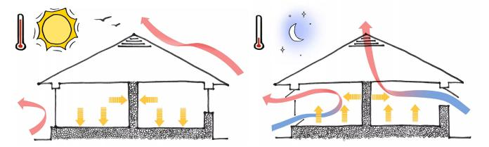
Figure #11-1: Illustration of thermal mass and night-time ventilation: Heat is absorbed during the day into high thermal mass elements; at night, the heat is released into the rooms and ventilation helps dissipate it to the outside.
