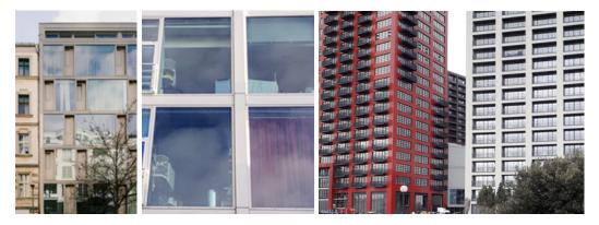
Figure #6-4: Examples of glazing proportion over 65% of facade area; (top) with partial shading through balconies and recesses; (bottom - Happy Facades) unmitigated. Note the left and middle examples show substantial use of internal blinds, likely to be for privacy and control of solar gains
