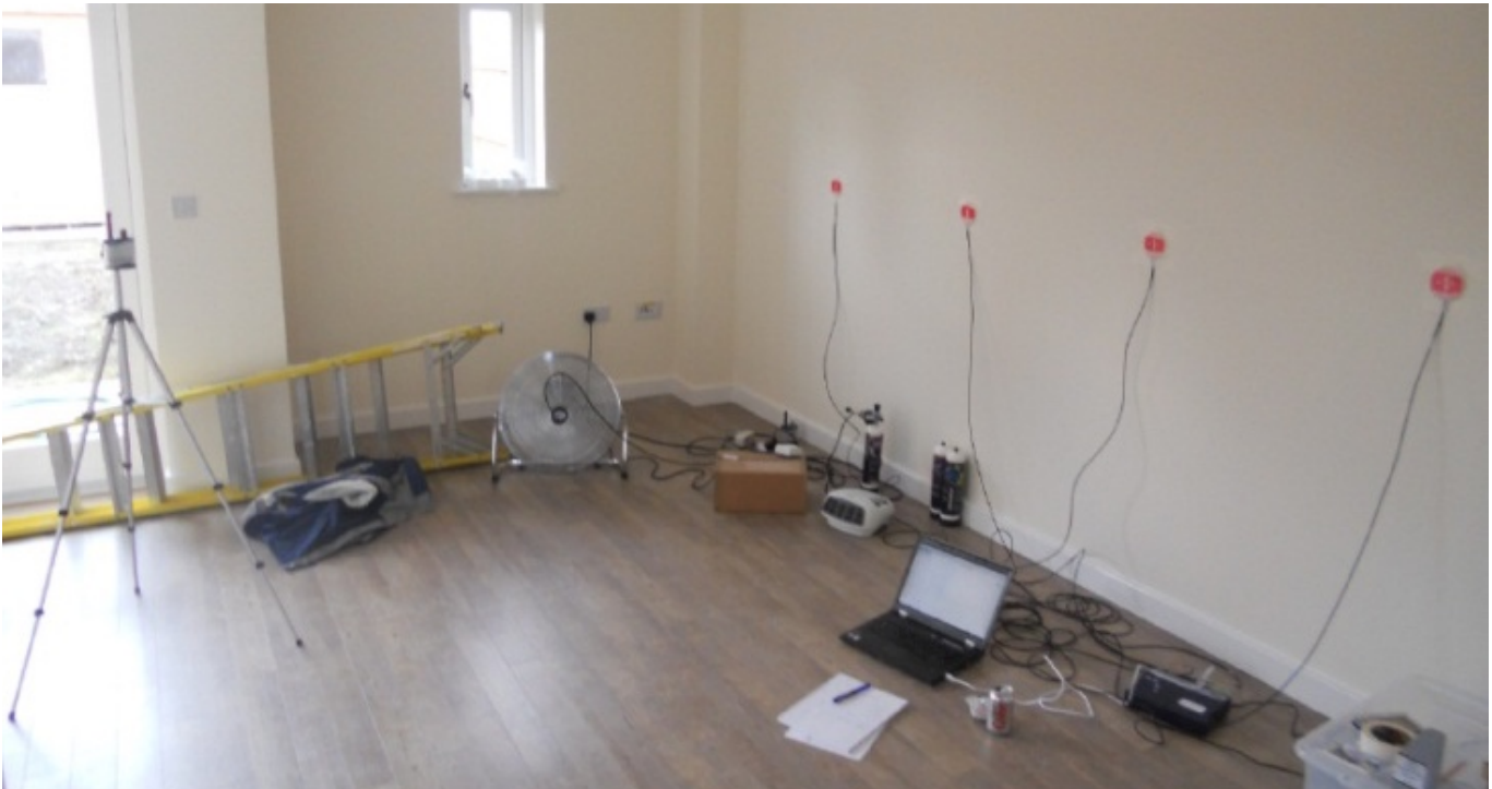
Figure 2. Heat flux sensors on walls (co-heating test instrumentation also shown)
